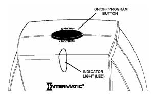
5. To manually turn OFF the **HA02 Appliance Module**, simply press and release the Program/ON/OFF button. The green indicator will turn OFF and the lamp or appliance plugged into the **HA02 Appliance Module** will also turn OFF.
