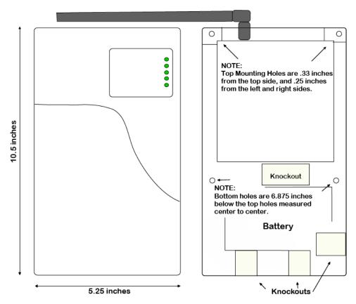
Figure 2: Inside & Outside Mounting Dimensions for the 2550
