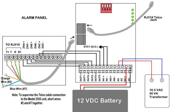
Figure 3: Connections Between the 2550 and the Alarm Panel
