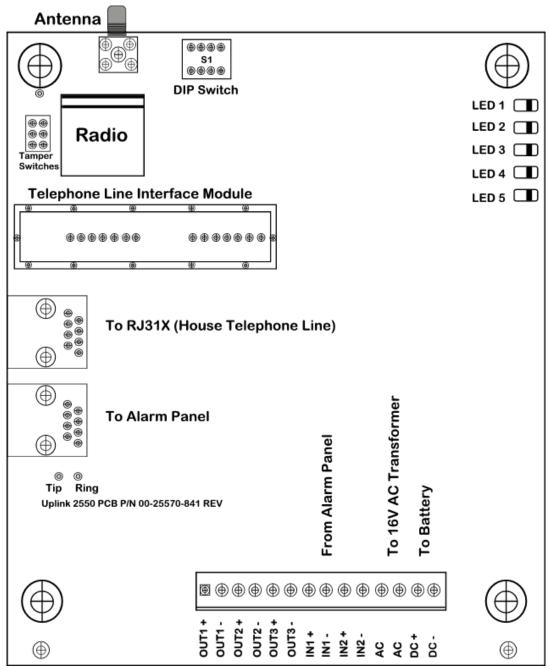
Figure 1: Parts on the 2550 PC Board
