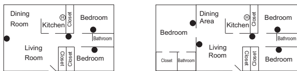
Figure 2 - Smoke Detector Placement
