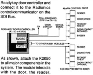
request to exit, the door controller, the door held open buzzer, the Radionics panel and one or more K2051 Access Prohibiter modules.
