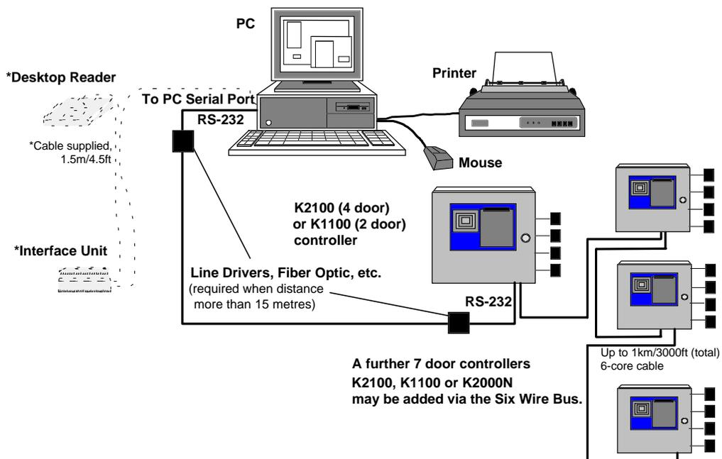
**Site Type 3. Site using Six Wire Bus from a Central Network Controller**
