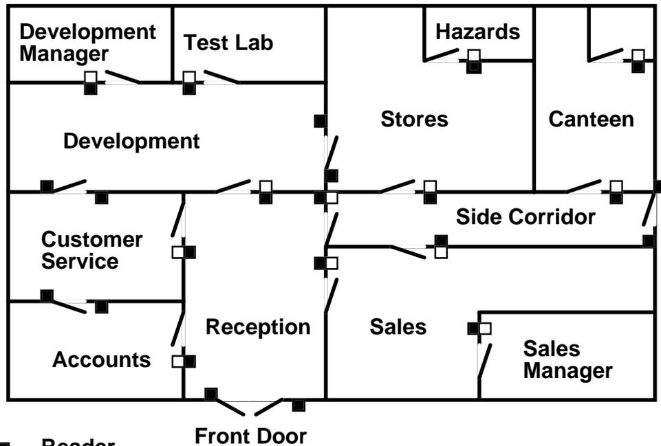
In this example you will notice that several doors have a **reader** on each side. This is to allow access to be controlled in both directions. For instance the door between Accounts and Customer Service has a reader on each side, this is because the same door is an entry door into both Accounts and Customer Service. Other doors have **Request to Exit (RTE)** motion detectors that allow any person to leave the area.
