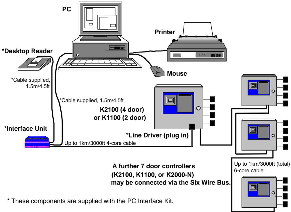
**Site Type 2. K2100 or K1100 Master Controller directly connected to PC**
