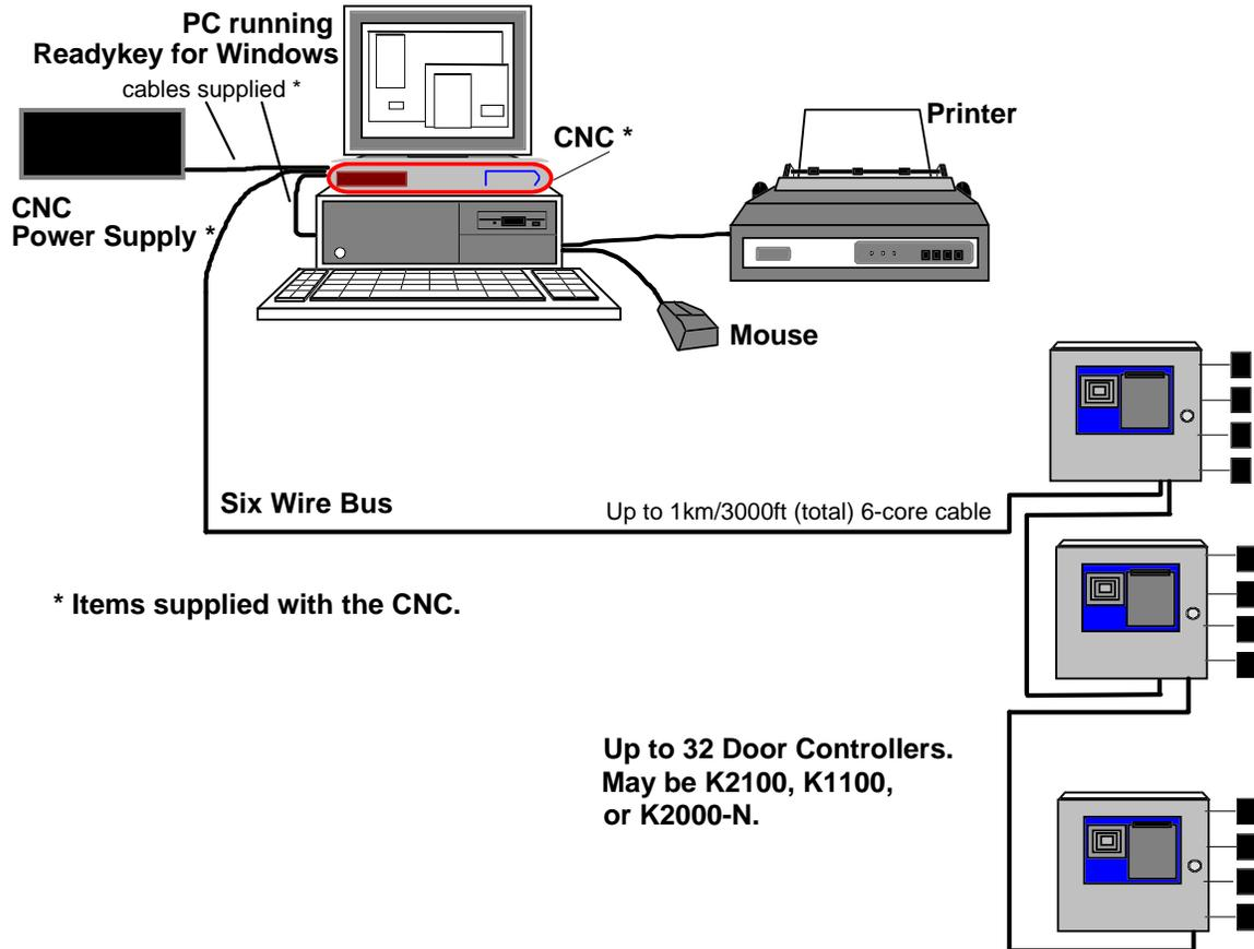
**Note:** It is possible to have as many as 4 CNCs on a single PC. However, each CNC requires one of the first four serial ports (COM1 - COM4) and each of the COM ports must have a separate IRQ number. Contact your computer hardware supplier for more information on COM ports and IRQ settings. If the COM ports are used for other equipment then this will reduce the possible number of CNCs.
