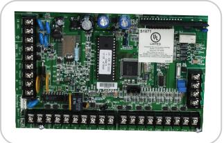
Control panel with 8 points expandable to 24, 4 outputs expandable to 12, 2 areas.
