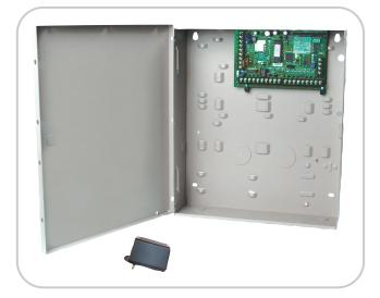
Control panel with 8 points expandable to 24, 4 outputs expandable to 12, 2 areas.
