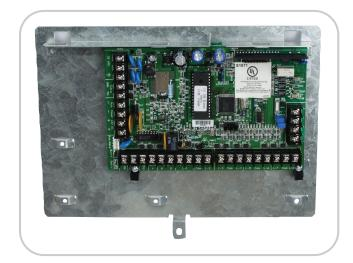
Control panel with 8 points expandable to 24, 4 outputs expandable to 12, 2 areas.
