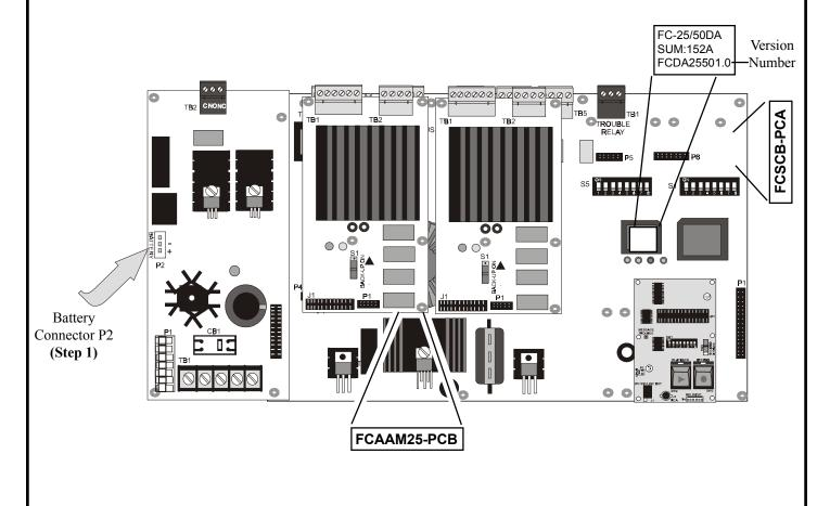
2. Unplug the field wiring terminal block from connector TB2 of the FC-PSM2 Power Supply Module. Remove and retain the four screws and washers from the corners of the module. Carefully unplug the FC-PSM2 module from the main circuit board and place it in the bottom of the cabinet. It is not necessary to disconnect the AC wiring (circuit breaker was turned off in Step 1) or transformer cable.
