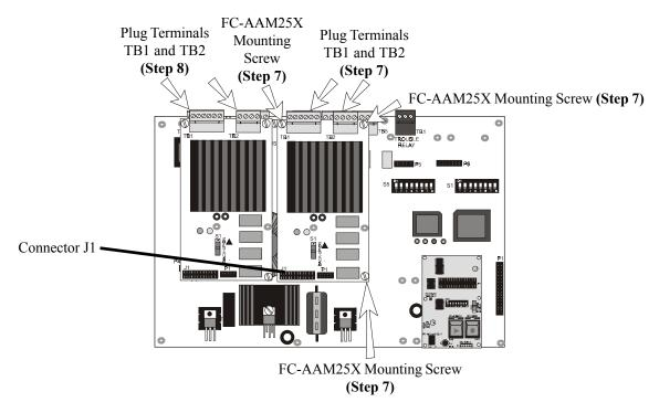
9. Install the FC-PSM2 module by carefully aligning connector P7 on the main circuit board with connector J1 on the FC-PSM2 module and pressing the module into place. Secure the FC-PSM2 to the four standoffs with screws and washers which were previously removed. Plug the field wiring terminal block into connector TB2 of the FC-PSM2 Power Supply Module.
