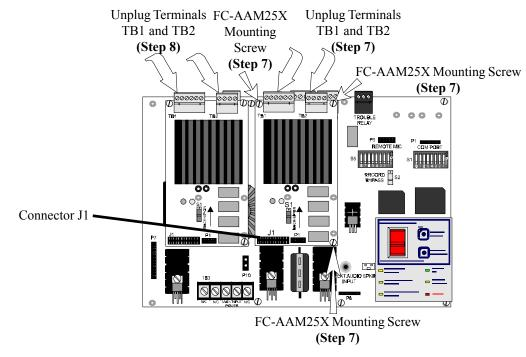
9. Install the FC-PSM(E) module by carefully aligning connector P7 on the main circuit board with connector J1 on the FC-PSM(E) module and pressing the module into place. Secure the FC-PSM(E) to the four standoffs with screws and washers which were previously removed. Plug the field wiring terminal block into connector TB2 of the optional FC-PSM(E) Power Supply Module.
