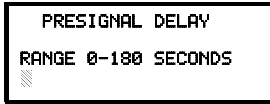
Pre-signal Delay Screen
