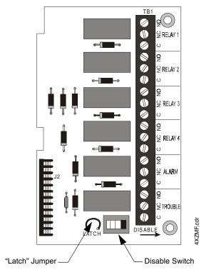
Figure 16 Wiring the Zone Relay Module
