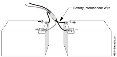
Figure 20 Battery Connections
