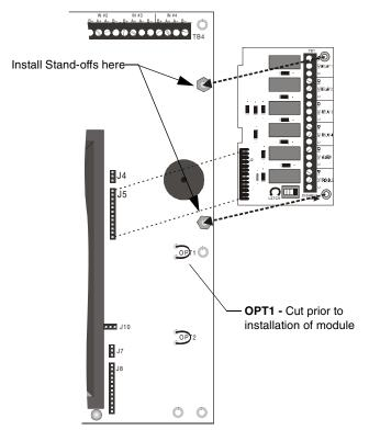
Figure 13 Module Installation - Upper Position
