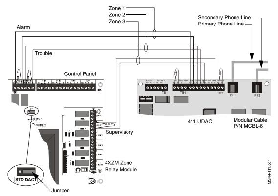
Figure 25 411UDAC Connections
