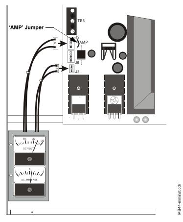
Figure 3 Mounting and Connecting the Meters
