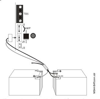
Figure 5 Battery Installation and Connection
