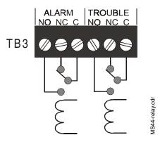
Figure 11 Schematic Representation of Alarm/Trouble Coils & Contacts
