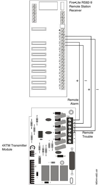
Figure 27 RS82-9 Connections
