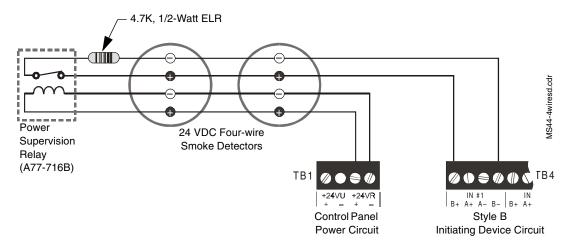
Figure 8 Typical Connection for Four-Wire Smoke Detectors
