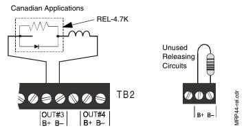
Figure 10 Releasing Circuits
