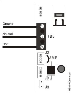
Figure 4 AC Power Connections
