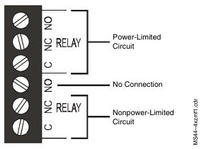
Figure 17 Mixing Power-Limited and Nonpower-Limited Circuits
