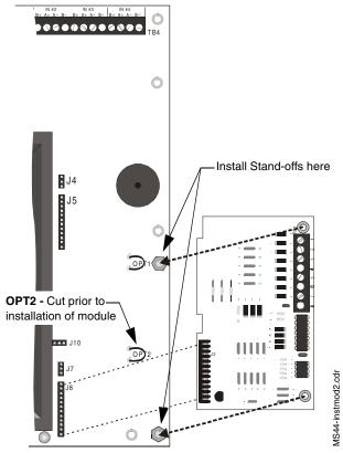
Figure 14 Module Installation - Lower Position
