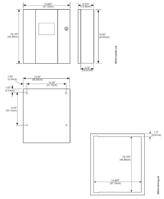
**Figure 2 Cabinet Mounting Dimensions**
