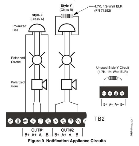
Output Circuits 2. Installation
