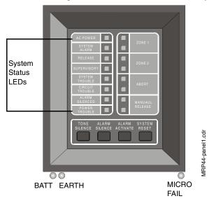
Figure 21 System Status LEDs
