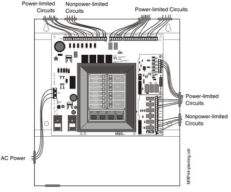
Figure 6 Power-limited Wiring Requirements
