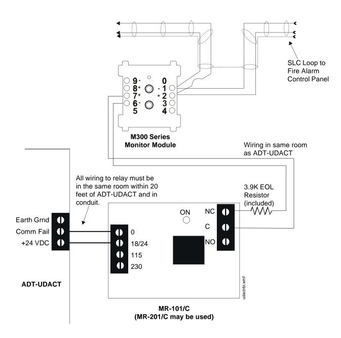
Note: M300 Series Monitor Module is used to supervise Normally Closed output of MR-101/C. On ADT-UDACT trouble and Comm Fail, MR-101/C relay contact will open causing the monitor module to transmit trouble condition to FACP.
