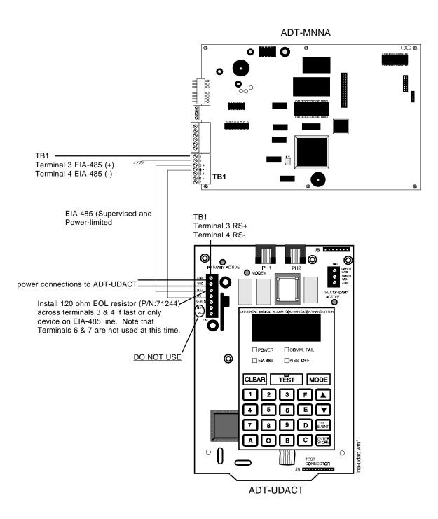
Figure F-1: EIA-485 Connection to Panel Mounted ADT-UDACT
