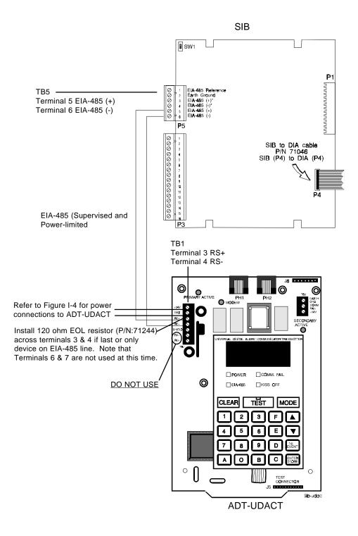
Figure D-3: EIA-485 Connection to Panel Mounted ADT-UDACT
