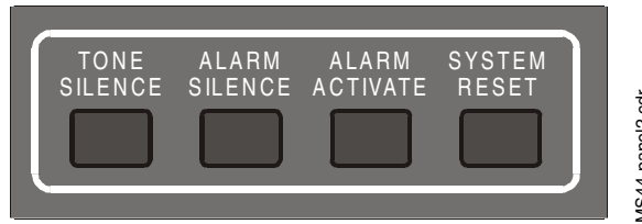
Figure 22 Control Panel Switches
