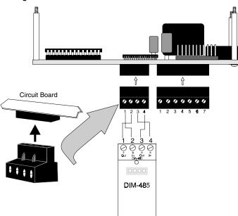
Figure 4-3: DIM-485 Connections
