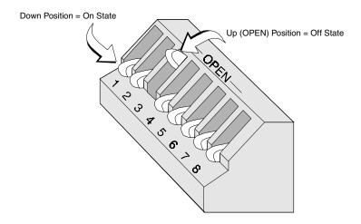
Note: SW1 DIP switch settings as illustrated in Figure 1-3 are as follows:
