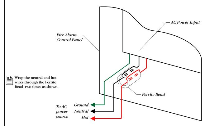
Installing a Ferrite Bead
