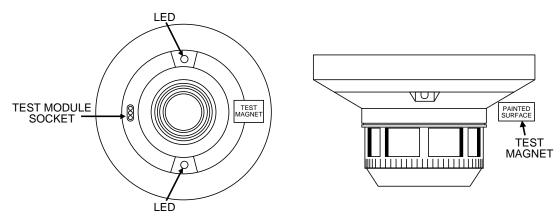
Figure 2. Views showing position of test magnet
