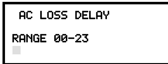
AC Loss Delay Screen #2
