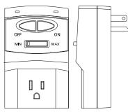
The HS-SP7670 Safety Plug plugs into any standard residential 120VAc electrical outlet to provide control over appliances rated up to 1500 watts maximum. The module's userselectable timer automatically turns off power to the appliance when the preset time has elapsed, ensuring that appliances are not left on for long periods of time without supervision. The appliance may be turned ON or OFF manually using the buttons on the Safety Plug.
