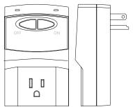
The HS-LM7500 lamp dimmer module is a device that plugs into any standard residential 120VAc electrical outlet to give you complete On, Off and dimming control of any incandescent lamp rated up to 300 watts maximum. The HS-LM7500 is CEBus-compliant (CEBus is a registered trademark of EIA), allowing for remote control of the module using CEBus spread spectrum powerline communications protocol. The module also supports directed address acquisition for Home Plug-and-Play (HPnP) installations.
