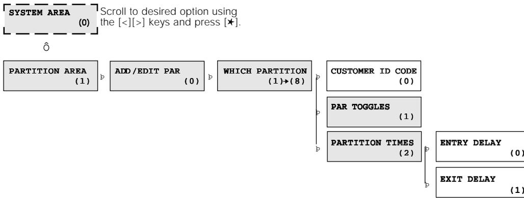
Using the first method the arrow keys would have to be pressed many times to scroll to the various items followed by the [★] key to select the item. Twelve keystrokes would be required after entering Installer Programming providing no mistakes are made. The keystrokes required are as follows:
