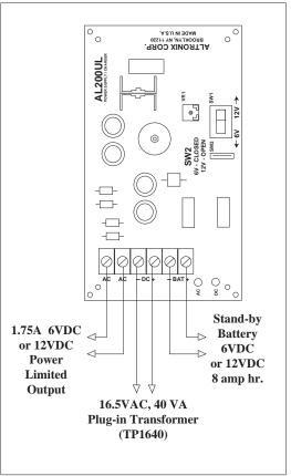
applied, if not the transformer's internal fuse could be blown and the transformer (16.5VAC/40VA UL Listed transformer) must be replaced.
