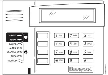
Figure 1: 6160CR-2 Key Functions for Programming the Communicator
