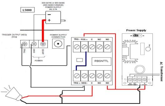
Due to the 3mA current limit of the L5000 output trigger, the Altronix TTL Sensitive relay must be used. A jumper wire is required from TRG+ to the POS+ terminal, as well as a common ground.
