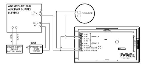
2. If you can get a wire from the L5000 to where you want the sounder you can use this setup: (An <u>Altronix RBSN-TTL</u> relay and power supply are required)
