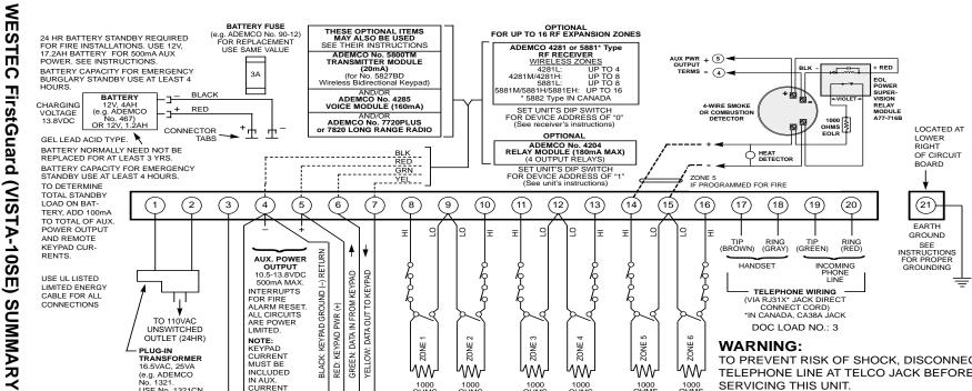
CONNECTION OF THE FIRE ALARM SIGNAL TO A FIRE ALARM HEADQUARTERS OR A CENTRAL STATION SHALL BE PERMITTED ONLY WITH THE PERMISSION OF THE LOCAL AUTHORITY HAVING JURISDICTION. THE BURGLAR ALARM SIGNAL SHALL NOT BE CONNECTED TO A POLICE EMERGENCY NUMBER.
