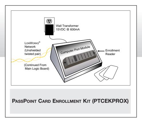
The enrollment kit has everything you'll need to equip your PassPoint Access Control System with card enrollment capabilities. This optional kit is a unique feature of Passpoint Systems and allows batch enrollment of cards. Card numbers are logged in the system by merely presenting the deck of cards to the enrollment reader.
