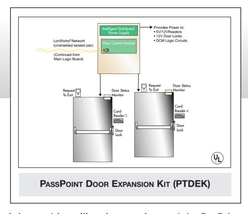
Your expansion kit includes materials you'll need to expand your existing PassPoint Access Control System. Each single kit provides the basic equipment for an additional one or two-door installation.
